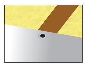
Temporary attachment is then made about 30mm from the upper edge of the lap joint by means of suitable BS 5534 fixings. Battens or counter battens are fixed permanently later on during the installation process.
