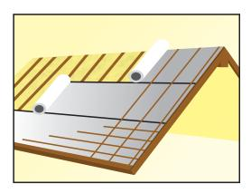
This insulated roof underlay product is a laminate made from a low emissivity reflective membrane and white polyester insulation. The reflective side should be installed facing to the outside of the construction. The first layer should be unrolled parallel to the bottom of the roof. The lap joint with the integral adhesive tape strip always faces down.
