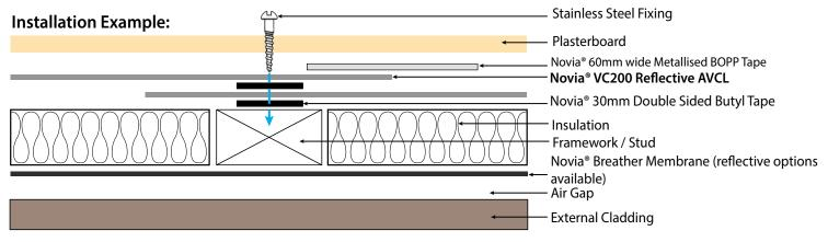
Please note - this diagram is not to scale and should only be used as guidance for the installation.
